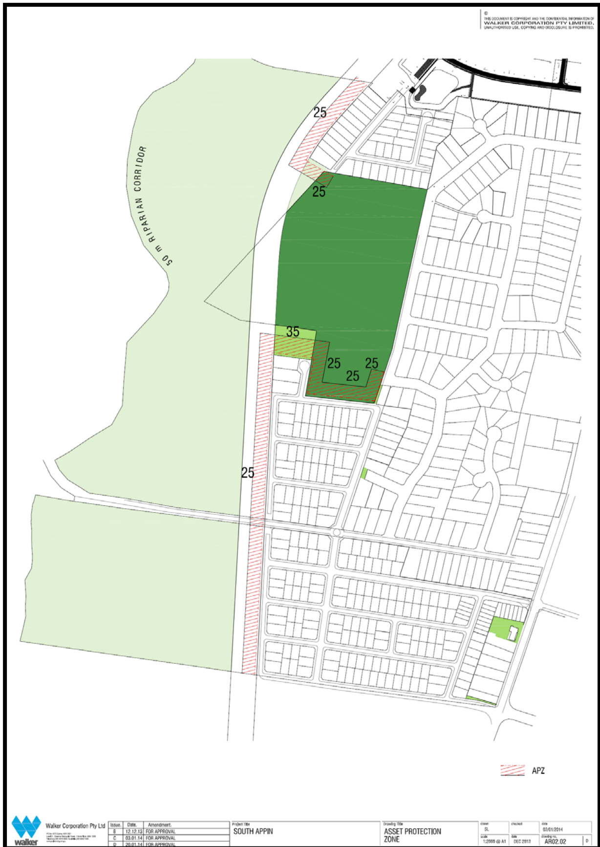
Figure 8: plan showing APZs complying with PBP-2006 Appendix 2
