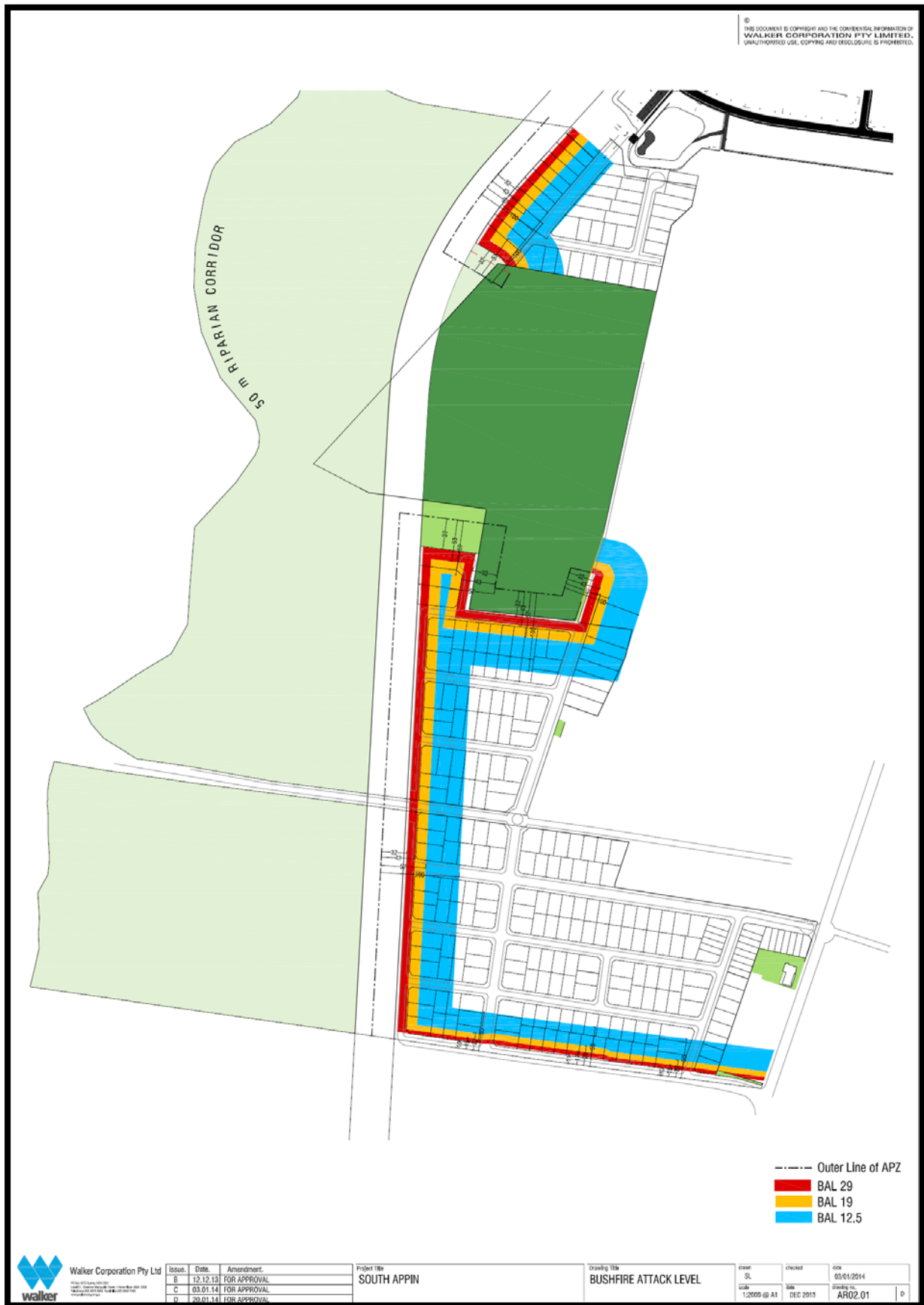
Figure 12: plan showing BAL thresholds – AS3959-2009
